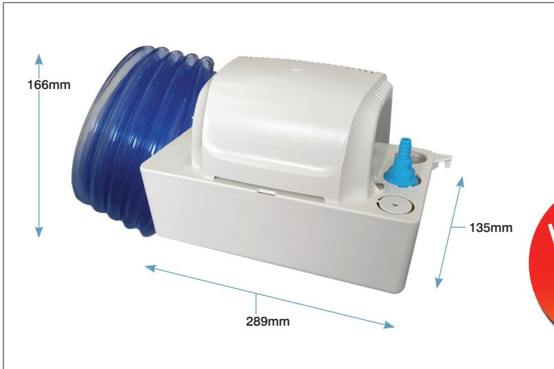
This Pump House compact 2 litre pump has an impressive 5.5 metre discharge lift. It can be floor or wall mounted and comes with a quick release check valve. Suitable for boilers up to 200kW, this pump comes with 6 metres of 9.5mm (3/8") ID flexible hose.
